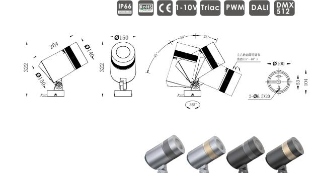
Left or right rotate the rotary ring to adjust focusing to adjust beam angle available from 15°~60°
